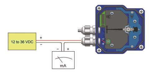
The connection is made in the terminal block. The positive terminal of the power supply is connected to the position + and the positive terminal of the load in the position -. The negative terminals of the power supply and the load are connected together. The instrument works in a 2-wire system, that is, the supply and signal line is the same. It is recommended to use a twisted pair wiring or shielded cable to avoid interferences in the current loop.
